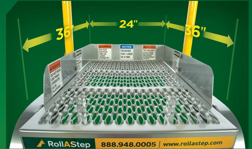
Six square feet of work area is roomy enough for an operator, tools and parts.
