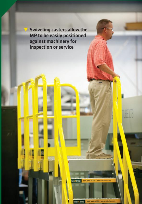
▼ Swiveling casters allow the MP to be easily positioned against machinery for inspection or service
